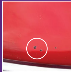
Bonnet Paint Chip Damage
