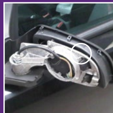
Missing Mirror Cover
