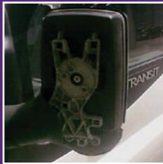
Missing mirror cover
