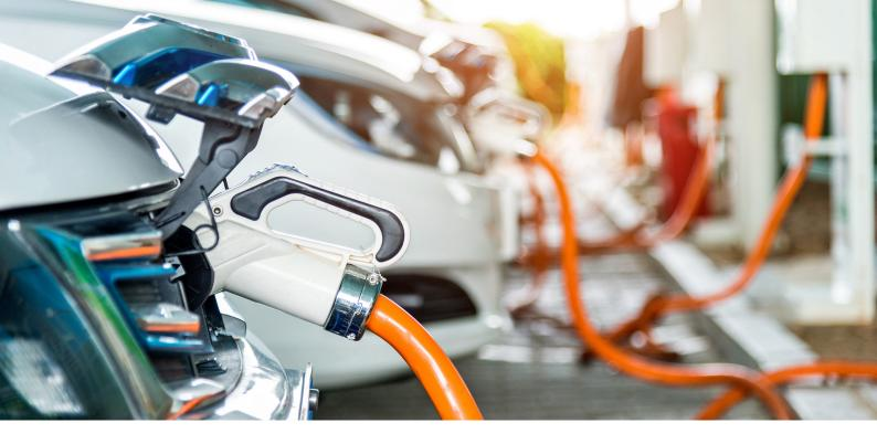
When thinking of chargers, you will need to consider if you prefer them to be "tethered" (i.e. with a cable permanently attached) or "untethered" (i.e. with the cable kept separately, most likely in the boot of the driver's vehicle.) A tethered charger is convenient and fast, while an untethered cable means you can swap the cable to suit different connectors, although the vast majority of electric cars use Type 2 connectors.
